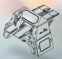
The machine is fully manufactured in stainless steel and food grade materials. Driven by Curio Stainless Steel water cooled motors.
